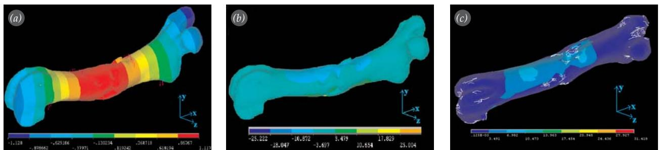
**Fig. 4.** (a) Deformation distribution in the loading area in a rat femur, (b) strain distribution after the loading, and (c) Von Mises strain distribution.
