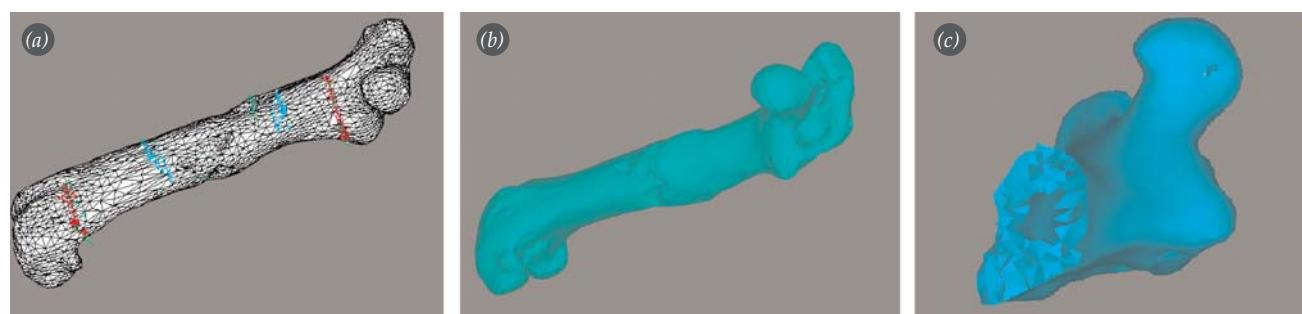
**Fig. 3.** (a) The elements formed for the analysis and loading areas for 4-point bend test, (b) generated femur model, and (c) sectional view of the femur model.
