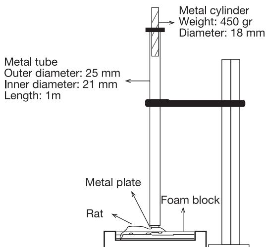
**Fig. 1.** Diagram of the head trauma induction system.
